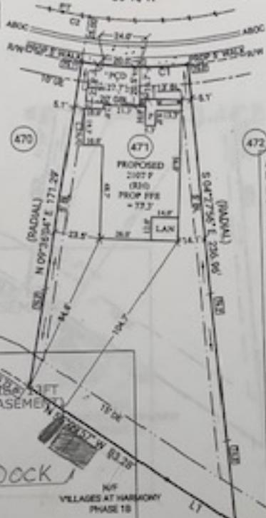
All new permit submittals for home sites will require proposed mechanical equipment to be located 10' away from any existing equipment on adjacent lots. This is to show compliance with our LDC (ch 3.2.2.E.8) which requires 10' between equipment that can affect access or drainage. Site plan should show the drainage plan proposed for the new site and how it will tie into the existing adjacent grade (include swales, water flow direction, and street, sidewalks, drives, house, and finish grade).
